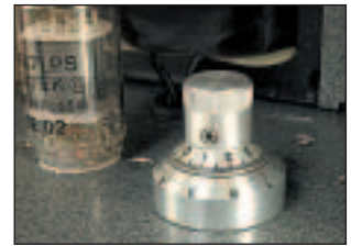
Swapping tubes is easy, thanks to the test-point jacks and the precise, 10-turn bias pot.
